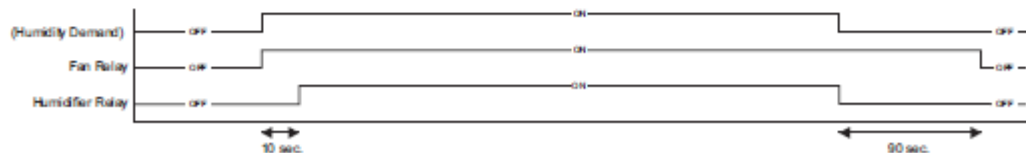
Humidistat - Relay Timing Chart
